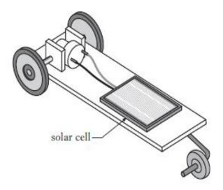
The solar cell produces a voltage of 0.5 V and a current of 0.4 mA.
